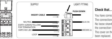
You have correctly identified the wires. The connections are tight. No loose strands have been left out of the connection block. The cover on the connection box has been replaced.
