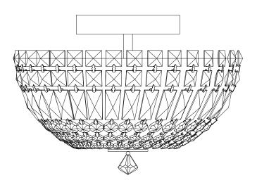
Voltage: 230V - 50/60Hz Lampholder: G9 Lamps: 3 x 33W Max
