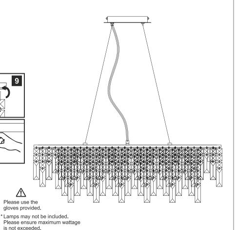
Voltage: 230V - 50/60Hz Lampholder: G9 Lamps: 6 x 33W Max
